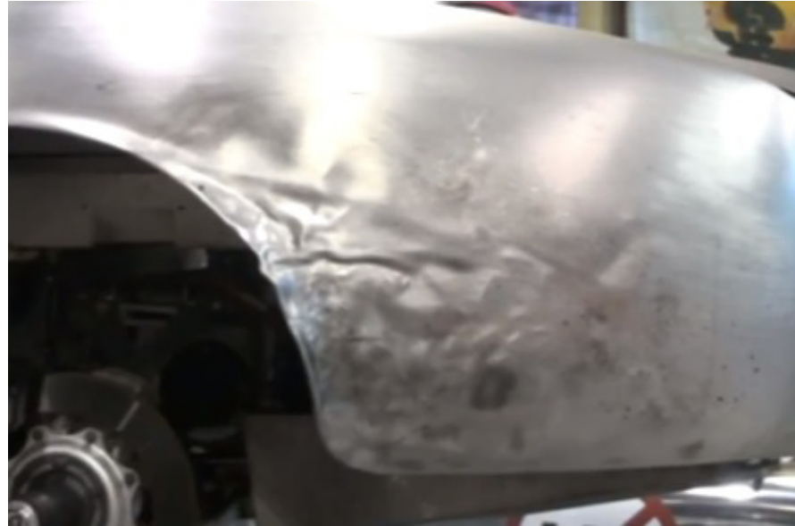
Before work on wrinkle
